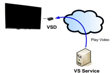
4. The Video Streamer Device streams the video from its source (such as the Internet) and because it is connected to a monitor, the video appears on that monitor.
