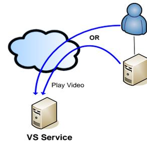
3. The central Video Streamer Service commands the Video Streamer Device to play a video stream, via its already established network connection. No new inbound connection is required.
