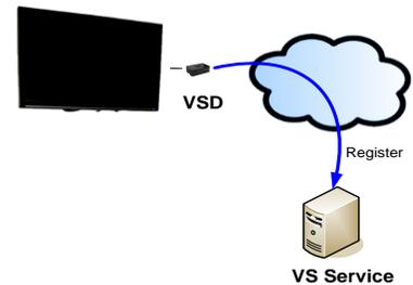
2. The user, via our web-based user interface, **or** via your system (if integrated), selects the video to be displayed on a monitor, and our software (or yours) sends a command to the Video Streamer Service identifying the monitor and video stream.
